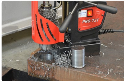
Milling capacity up to 70 mm (2-3/4") • Max depth up to 75 mm (3")
